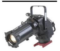
A base down axial profile delivering a "cool" beam of light in a range of fixed beams including 20°, 30°, 40° and 50°. The beam is of crisp "white" light with little or no distortion, ideal for pattern projection and precise beam shaping.
